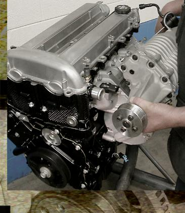
**123.** The stock supercharger can make the 300 hp and needs to be installed with the factory 8 mm bolts and studs torqued to 18 ft-lbs. The pulley will need to be replaced with a smaller unit to take advantage of the new performance camshaft, valvesprings, pistons and fuel injectors.
