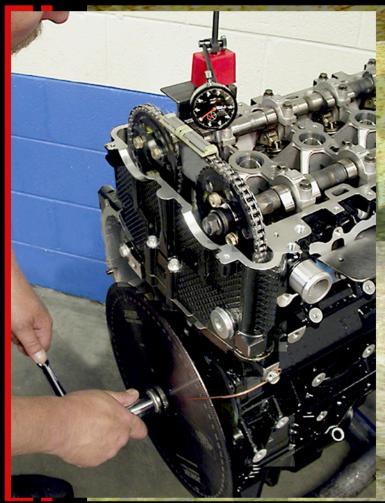
105. Move the valve height dial gauge to an exhaust valve on the No. 1 cylinder and repeat the process of determining TDC, zeroing the gauges and degree wheel and running through 0.050 inch lift at before TDC and after TDC, recording the degree wheel location at each point.
