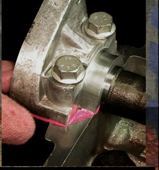
109. It is important to completely wipe off any sealer that is forced out of the mating point between the cap and cylinder head to avoid it getting into the engine oiling system.
