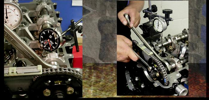
**104.** The intake cam was supposed to be centered at 102 degrees on the crankshaft. The 0.050 inch lift numbers were 136 degrees and 69.5 degrees. Adding these together and dividing the sum by 2, equaled 102.25—which for most engine builders would be called 102 degrees.
