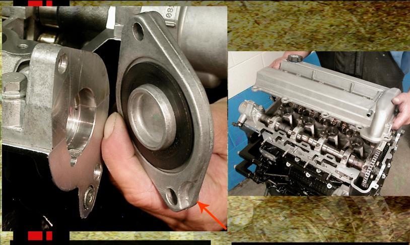
114. The rear cam cover plate on the intake cam side needs to be installed with the notch in the face of the cover (arrow) located near the bottom bolt. This is to clear the Allen head bolt in the block—if you don't do this, the plate will leak profusely on startup of the engine! Torque the two 13 mm bolts to 10 ft-lbs.
