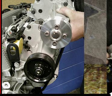
**124.** The new GMPP 73 mm pulley increases the RPM of the blower vanes, which increases the inlet air boost to the engine. It is installed by removing the bolt holding the stock pulley in place, using a pulley puller on the stock pulley and pressing the pulley on with a pulley installer. Torque the holddown bolts to 16 ft-lbs after applying one drop of red Loctite to the threads.
