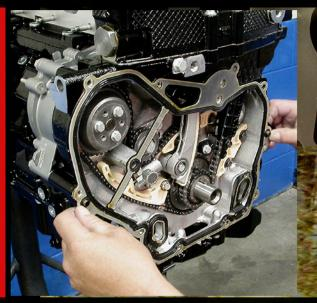
**116.**Position compression-style front cover gasket on the dowels protruding from the block in preparation for installing the cover.
