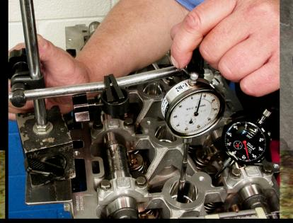
**100.**On the No. 1 cylinder, install the dial gauge so its plunger reaches down through the spark plug hole to touch to top of the piston. The other dial bore gauge plunger should rest on a retainer of one of the No. 1 cylinder intake valves. Align both gauges so the plungers are 'in line' with the stroke of the piston or valve—so their measurements are accurate.
