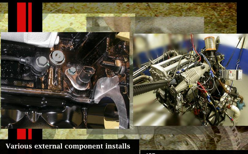
**126.**On the intake cam side of the engine block, torque the crank location sensor to 18 ft-lbs, and engine knock sensor to 89 in-lbs.
