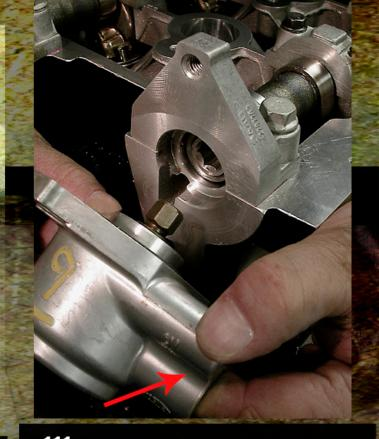
As you can see, there is a male and female hex engagement that must go together. To get the sensor wheel installed correctly, place the notch in the 4 o-clock position (arrow) when looking at the wheel body from the back of the engine. Make sure the engine is on the No. 1 piston's compression stroke and slide it onto the hex drive gear coming off the exhaust camshaft.
