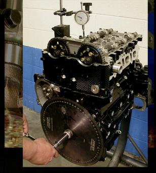
**97.** Install degree wheel on snout of crank. A large degree wheel needs to be acquired for this activity. Bolt it handtight (*for now*) to the snout of the crankshaft.
