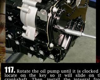
117. Rotate the oil pump until it is clocked to locate on the key so it will slide on the crankshaft. Then, install the integral front cover/oil pump over the gasket and locate it on the dowels. Install the front cover bolts to hand tight and install the final water pump bolt to hand tight. Now torque the front cover bolts down to 10 ft-lbs in a radial pattern and install the water pump bolt to 12 ft-lbs.
