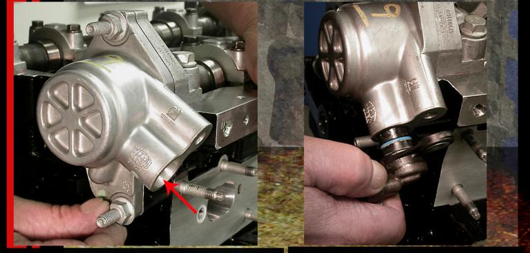
**112.** The stud/bolts holding the cam sensor body on the head should be torqued to 10 ft-lbs with a drop of red Loctite on their threads. You should be able to see the notch by looking up the hole for the sensor. (*arrow*)
