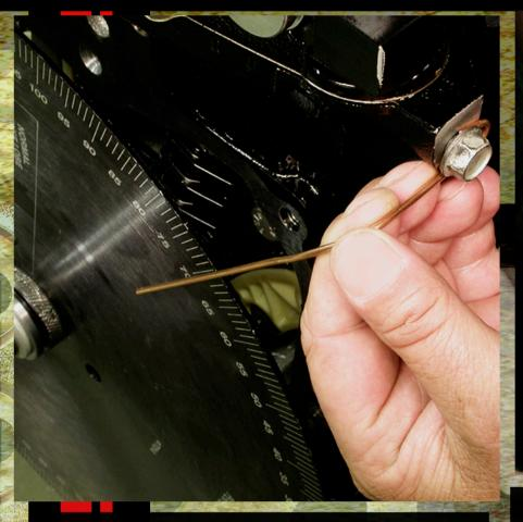
**98.**Create a wire 'pointer' and mount it firmly on the engine block. The end needs to be placed close to the surface of the degree wheel face so the numbers can be read clearly without variation.
