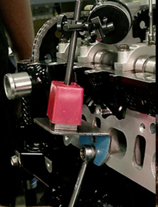
Two dial gauges with stands will also be needed to measure the piston location and valve locations. Simple angle-iron mounts with a hole drilled into one of them work great—mount them on the side of the head and affix the dial bore gauges to these with their magnetic bases.
