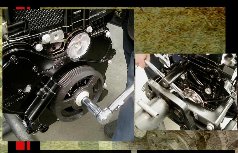
**116.** Slide the integral harmonic balancer/front pulley on the crank with its pointer located on the TDC position (this will allow it to mate with the oil pump drive) and torque the NEW bolt (GM pn 11589123) to 76 ft-lb (100Nm) and twist 125 degrees (+/-4 degrees). Apply engine oil to the bolt threads before installing.
