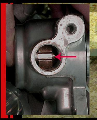
**110.** A key step that needs to be carefully completed is the installation of the cam sensor wheel and body. This notch (*arrow*) is read by the sensor to indicate where the engine is in its firing order, so it is critical to get it installed on the hex gear drive in the properly clocked location.
