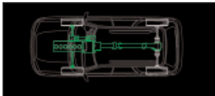
Longitudinally-mounted, in-line, 6-cylinder engine with 4WD system
